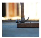
When the user of the hammer pushes down on the handle, the claw of the hammer pulls up on the nail. The hammer changes the direction of the force. It also applies greater force over a smaller distance.
