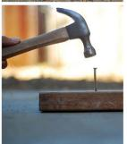
When a carpenter moves the handle of the hammer back and forth a short distance with strong force, the head of the hammer moves a greater distance back and forth against the nail but with less force. By repeatedly hitting the nail, the hammer drives the nail into the board.
